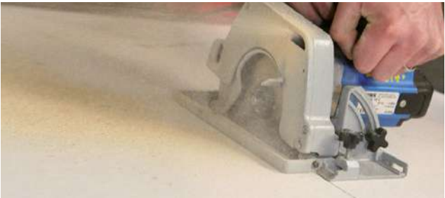
Picture No. 4: Cutting feed slower then for solid wood.
